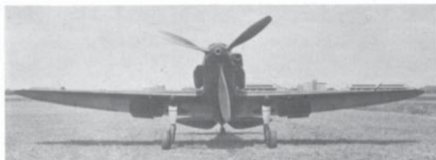
Above: the RE 2001 bis (MM.408, a modified RE 2000 prototype) with a redesigned wing, which reached 600 km/h but was not produced in series. Right: an RE 2001CN Falco II Serie IV (MM.90000) with exhaust flame dampers, 20 mm Mauser MG151 wing guns, a belly shackle for a bomb weighing up to 250 kg, painted entirely in semi-gloss black.
